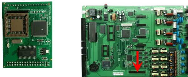
Figure 14: CO line and key-phone Extension installation
